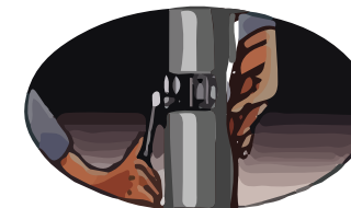
5. Screw both ends firmly, ensuring that both plates are parallel
