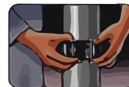
4. Lay collar around sealing
